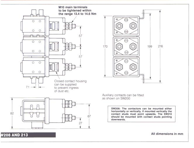
l-in voltages are approximately 6 and 66% of the rated voltage intermittent and continuously d types respectively.
