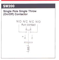
Single Pole Single Throw (Off/On) Normally Closed Contactor
