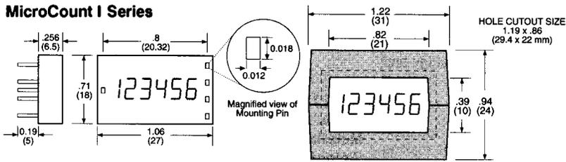
adaptor clips into panel .050 to .125 thick
