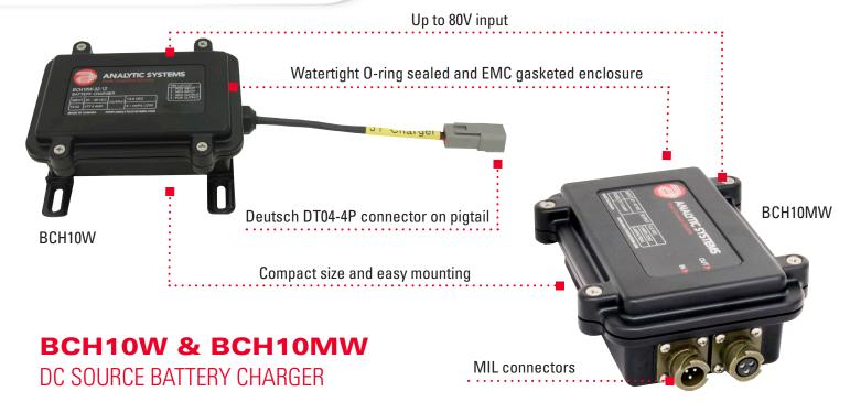
The BCH10 Step Down series of Battery Chargers supply up to 10 amps of charging current at 12, 24, 36 or 48 volts from any higher voltage between 20 and 80 volts DC in an IP66 rated watertight and EMC shielded enclosure for use in automotive, heavy equipment, marine, industrial, rail or alternative energy environments. The output voltage is configured to allow permanent connection to the battery.
